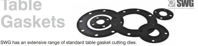
We cut standard table, ANSI, ASA, AS4087 and BS4504 gaskets in materials to suit customer needs, we use insertion rubber, EPDM, neoprene, nitrile, non asbestos including Shell and Waterworks approved materials plus other materials as specified and in the quantity required.
